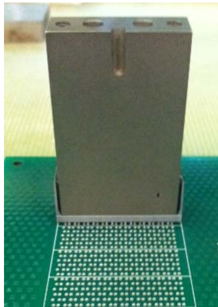
Figure 6: Ensure the cavities in the seating head match up to the blades on the backplane module.
