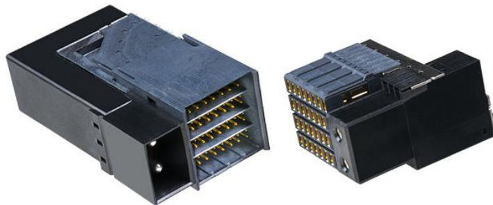
Figure 5: Example of Paladin direct orthogonal (left) and traditional daughtercard (right) with integrated power.
