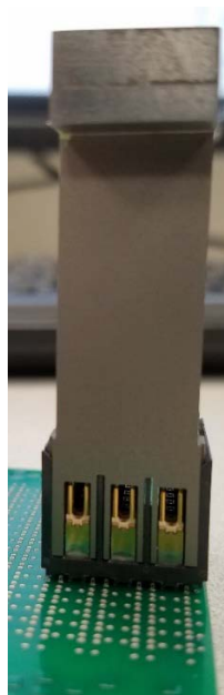
Figure 10: Proper 3 Pair loading head with 3x8 BMA module.
