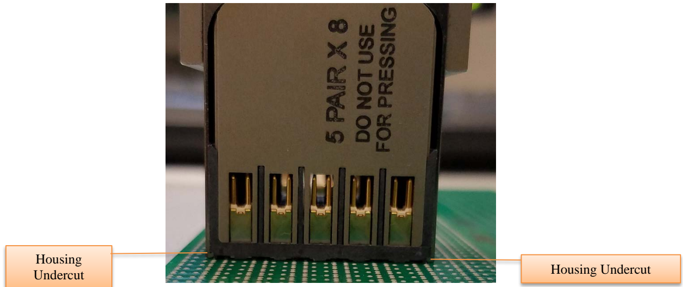
Figure 5: Removal module tool snapping over housing undercut.
