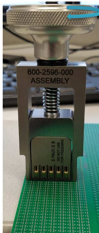
Figure 6: Twisting of knob for BMA module removal.
