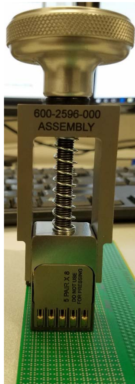
Figure 4: 5x8 BMA Module with insert block and clamp for removal.
